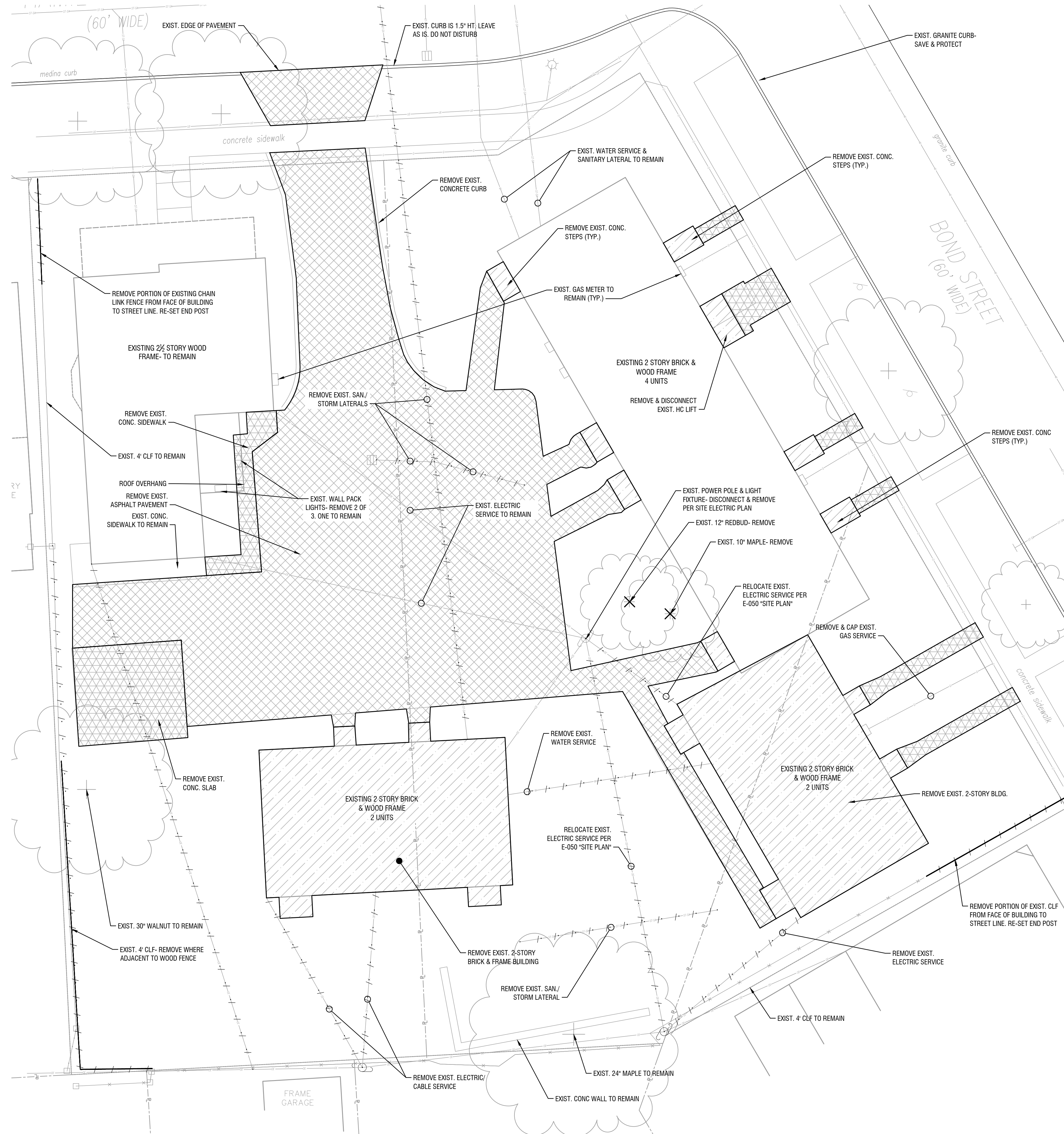
1 EXISTING CONDITIONS AND DEMOLITION PLAN SCALE: 1" = 10'
